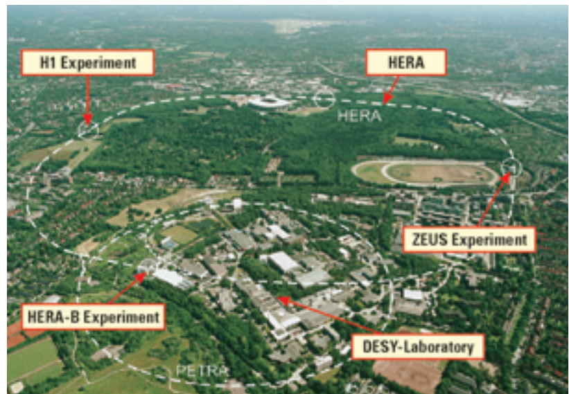
Fig. 3 Aerial view of DESY with the HERA accelerator (underground) indicated by the dashed line. The location of the two e-p collision experiments H1 and ZEUS (also under ground) is indicated as well as the location of the HERA-B Experiment, where proton-nucleus scattering is investigated (see [7]). (Source: DESY-PR)
