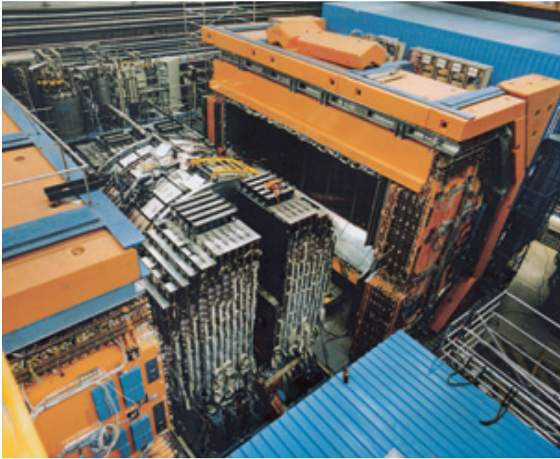
Fig. 4 View into the ZEUS detector which is opened for maintenance. The »heart« of this detector is the high precision Uranium-Scintillator Calorimeter (black device in the centre). (Source: DESY-PR)
