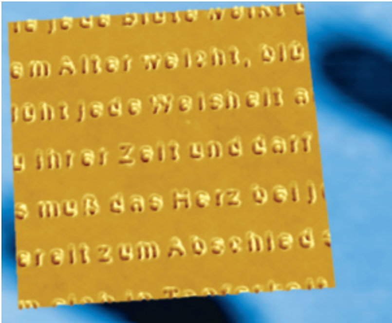
Fig. 4 Foreground: Written poem in PMMA by the DSM technique (Hermann Hesse, Stages , from The Glass Bead Game ), scan range 1.6 \times 1.6 \mu\text{m}^2 , height 26 nm. Background: SFM image of a compact disk, scan range 2.53 \times 1.95 \mu\text{m}^2 , height 243 nm. Foreground and background have the same scale. The storage capacity which can be achieved by the DSM technique is remarkably high. The dimensions of one letter are about 50 \times 100 \text{ nm}^2 .
